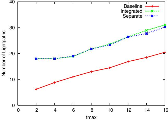
Fig. 3. Number of lightpaths used by each grooming method for the 6-node topology of Figure 2(a)
