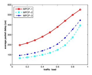
Fig. 4. Packet delay vs. traffic load, N = 16 and hot-spot traffic
