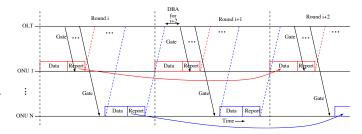
Fig. 2. The operation of MPCP-2 with look-ahead parameter  $\ell = 2$
