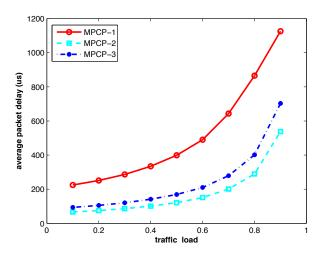
Fig. 3. Packet delay vs. traffic load, N = 16 and uniform traffic
