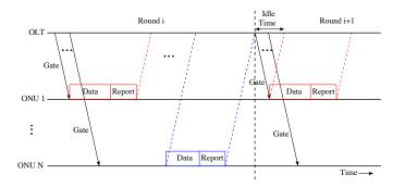
Fig. 1. The operation of the IPACT algorithm
