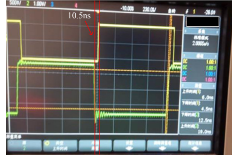
Fig. 16. Switching speed of the 4 \times 1 silicon photonic switch used for the tunable laser prototype.
