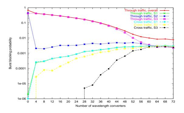
Figure 3.5: Burst blocking probability,  $T_{setup}(JIT) = 0.01, T_{OXC} = 1, \lambda = 0.15$
