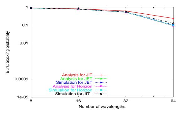
Figure 2.14: Single node performance comparison, Scenario 6 (distant future technology,  $1/\mu = T_{OXC}$ )
