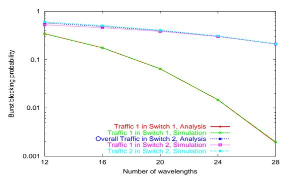
Figure 2.24: Simulation and Analytical result for a three-node OBS network,  $\lambda_1 = \lambda_2 = 16\mu$
