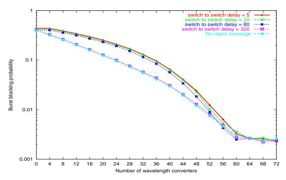
Figure 3.13: Through traffic burst blocking probability at switch  $S_3$ ,  $T_{setup}(JIT) = 0.01, T_{OXC} = 1, \lambda = 0.15$
