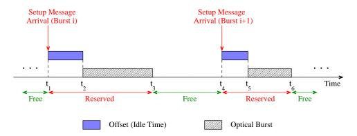
Figure 2.2: Operation and departure process of a wavelength with immediate reservation (JIT)
