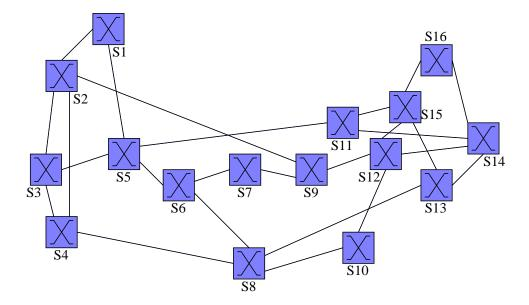
Figure 4.4: The 16-node topology based on the 14-node NSFNet
