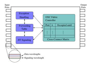
Figure 1.2: Logical diagram of the signaling engine at an OBS node
