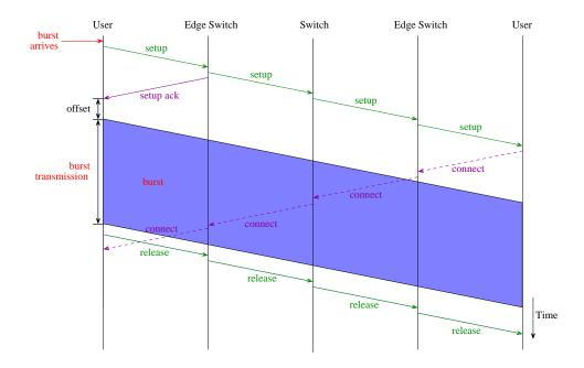
Figure 3.2: JumpStart JIT signaling messages in the OBS network for a successful burst transmission
