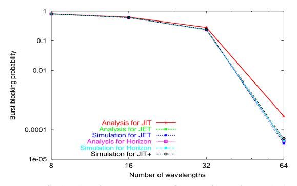
Figure 2.13: Single node performance comparison, Scenario 5 (distant future technology,  $1/\mu = 5T_{OXC}$ )
