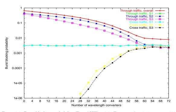
Figure 3.9: Burst blocking probability,  $T_{setup}(JIT) = 0.01, T_{OXC} = 1, \lambda = 0.15, \tau_{switch} = 320$
