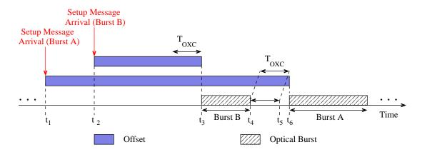
Figure 2.5: Non-FCFS service of a wavelength in an OBS node with delayed reservation and void filling (JET)
