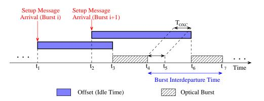
Figure 2.4: Departure process of a wavelength with delayed reservation and no void filling (Horizon)
