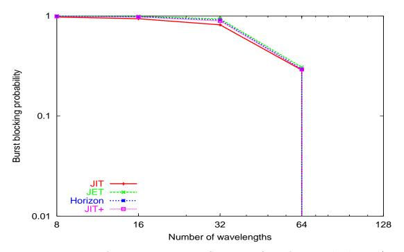
Figure 2.18: Path performance comparison, Scenario 3 (near future technology,  $1/\mu=5T_{OXC})$
