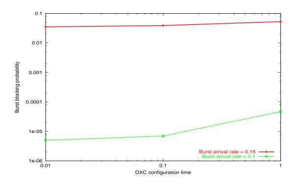
Figure 3.20: Burst drop probability of 4-hop paths, C = 100 converters
