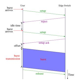
Figure 3.1: Signaling messages between a user and its edge switch in the JumpStart JIT protocol
