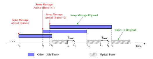
Figure 2.6: Operation of the modified immediate reservation scheme  $(JIT^+)$
