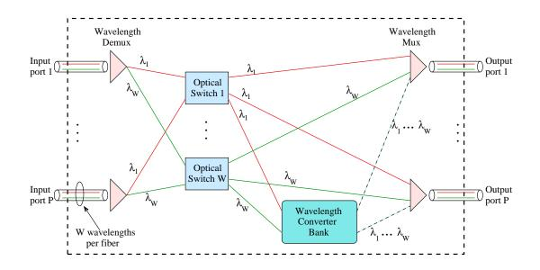
Figure 1.3: A  $P \times P$  OXC with a shared converter bank
