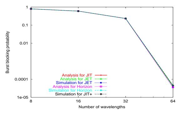
Figure 2.9: Single node performance comparison, Scenario 1 (current technology,  $1/\mu = 5T_{OXC}$ )
