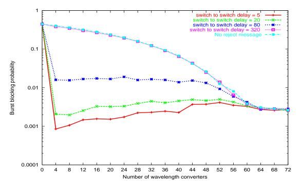
Figure 3.12: Through traffic burst blocking probability at switch  $S_2$ ,  $T_{setup}(JIT) = 0.01, T_{OXC} = 1, \lambda = 0.15$
