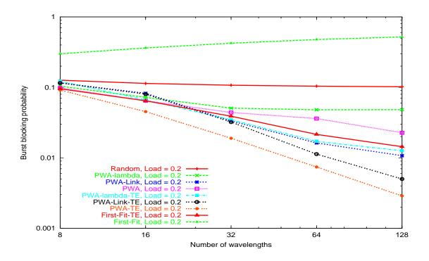
Figure 4.10: Burst blocking probability,  $4 \times 4$  torus network, load = 0.2
