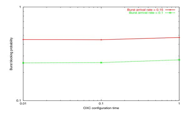
Figure 3.23: Burst drop probability of 5-hop paths, C = 4 converters
