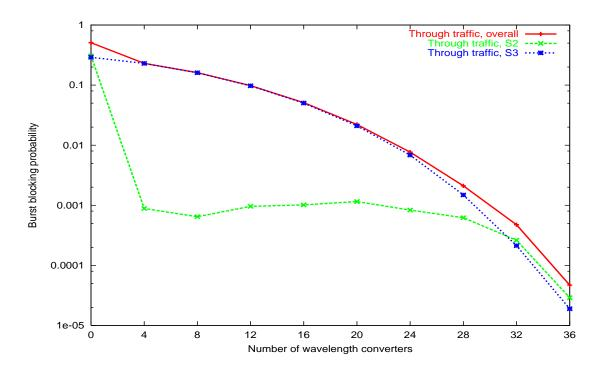
Figure 3.6: Burst blocking probability,  $T_{setup}(JIT) = 0.01, T_{OXC} = 1, \lambda = 0.1$
