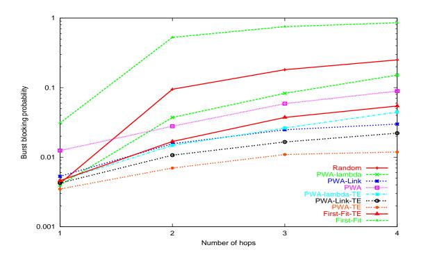
Figure 4.12: Burst blocking probability,  $4 \times 4$  torus network, load = 0.2, W = 64
