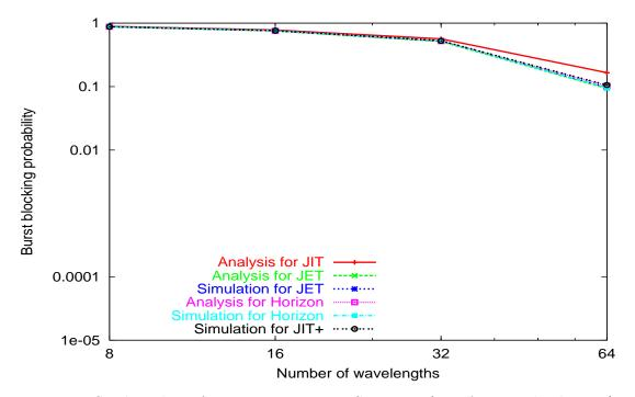
Figure 2.12: Single node performance comparison, Scenario 4 (near future technology,  $1/\mu = T_{OXC}$ )
