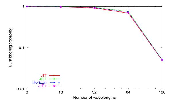
Figure 2.17: Path performance comparison, Scenario 2 (current technology,  $1/\mu = T_{OXC}$ )
