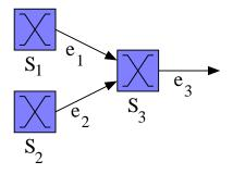
Figure 4.1: First-Fit results in high burst drop probability at Switch  $S_3$
