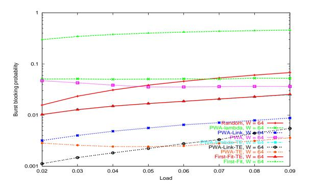
Figure 4.8: Burst drop probability, NSFNet, low load
