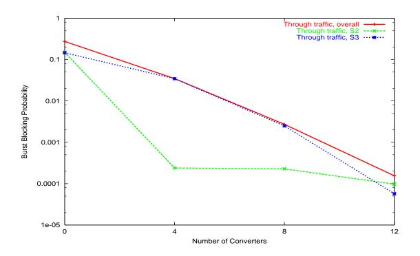
Figure 3.8: Burst blocking probability,  $T_{setup}(JIT) = 0.01, T_{OXC} = 1, \lambda = 0.05$
