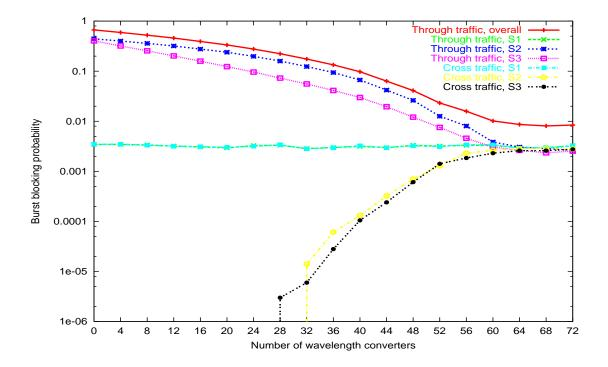
Figure 3.10: Burst blocking probability,  $T_{setup}(JIT)=0.01, T_{OXC}=1, \lambda=0.15$
