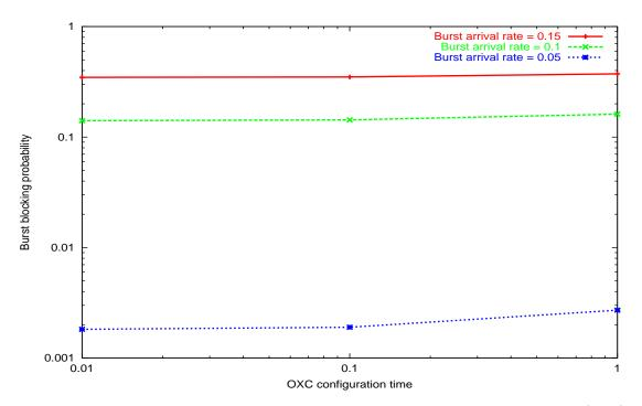
Figure 3.14: Overall through traffic burst drop probability, C = 8 converters,  $T_{setup}(JIT) = 0.01T_{OXC}$
