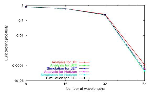
Figure 2.11: Single node performance comparison, Scenario 3 (near future technology,  $1/\mu = 5T_{OXC}$ )
