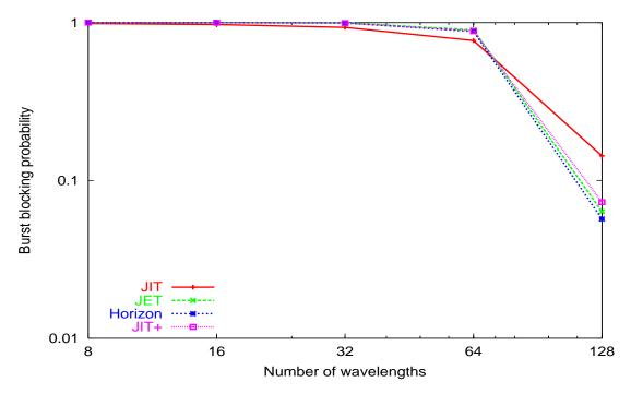
Figure 2.19: Path performance comparison, Scenario 4 (near future technology,  $1/\mu = T_{OXC}$ )
