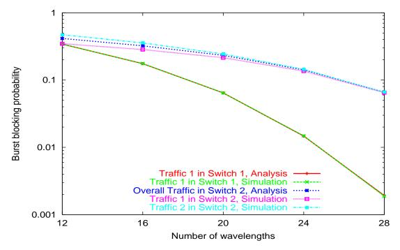
Figure 2.25: Simulation and Analytical result for a three-node OBS network,  $\lambda_1 = 16\mu$ ,  $\lambda_2 = 8\mu$
