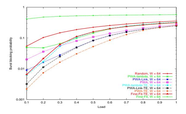
Figure 4.7: Burst drop probability  $4 \times 4$  torus network, moderate and high load
