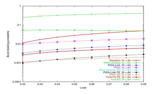
Figure 4.6: Burst drop probability,  $4 \times 4$  torus network, low load
