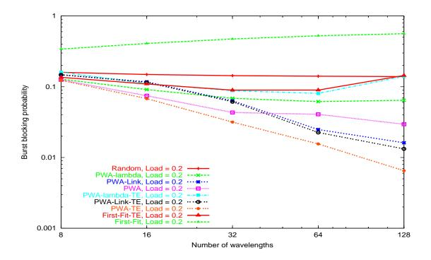
Figure 4.11: Burst blocking probability, NSFNet, load = 0.2
