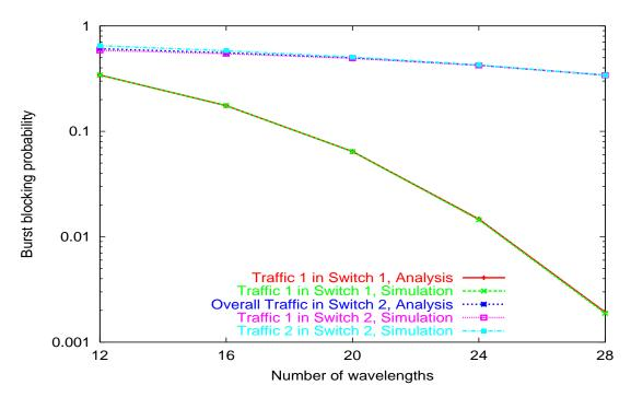
Figure 2.26: Simulation and Analytical result for a four-node OBS network,  $\lambda_1 = \lambda_2 = 16\mu$ ,  $\lambda_3 = 8\mu$
