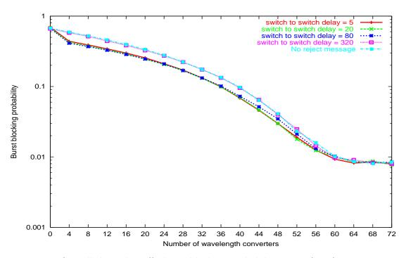
Figure 3.11: Overall through traffic burst blocking probability,  $T_{setup}(JIT)=0.01, T_{OXC}=1, \lambda=0.15$
