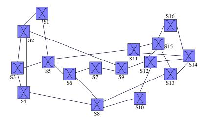
Figure 3.21: The 16-node topology based on the 14-node NSFNet
