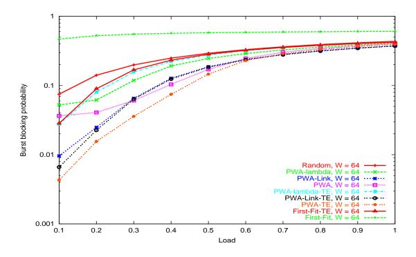
Figure 4.9: Burst drop probability, NSFNet, moderate and high load
