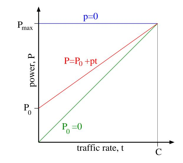
Most general model: minimize power consumption  $\rightarrow \min P$
